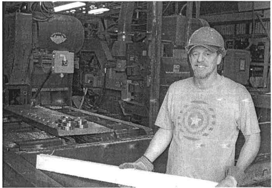
Brodie West inspecting finished precut stringers at the Brewer gang-saw outfeed belt before they are stacked for shipment.
