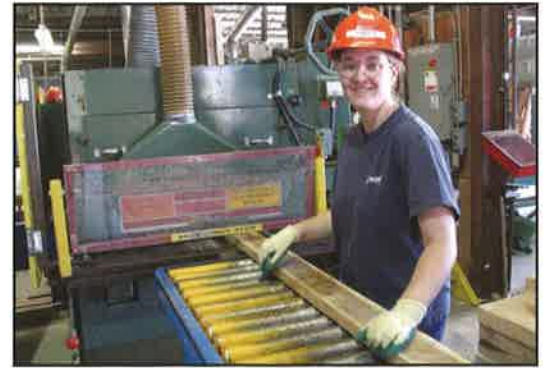
Amber Dean feeds lumber into a rip saw, which is one of the steps involved in manufacturing Townsend Lumber's patented Breeze Dried™ sticks that are used to separate lumber for air-drying.
